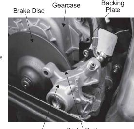
Brake Caliper Brake Pad Material
